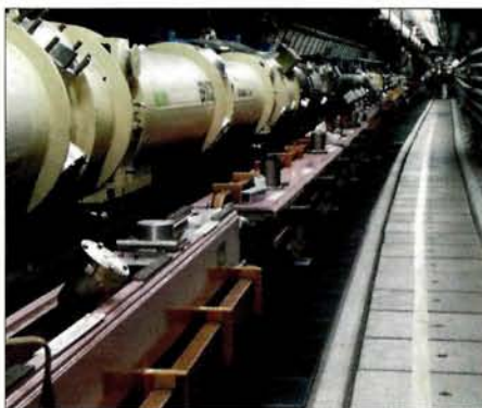
One of the two new spin rotator sections near the H1 detector, with a vertical dipole magnet in the foreground.
