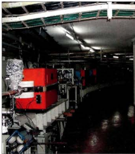
The BEPC machine will be upgraded to become a double-ring collider, with a luminosity 100 times higher than at present. (Mike Dykes, Daresbury Laboratory.)
